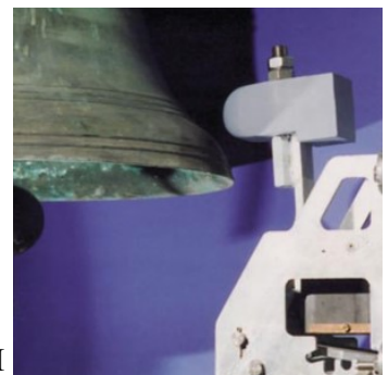
Fig. 6 Example of an externally mounted EMH
